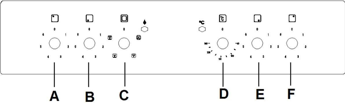
**A** Rear left cooking zone control knob ➤ Turn clockwise or anticlockwise to turn on the hob.
