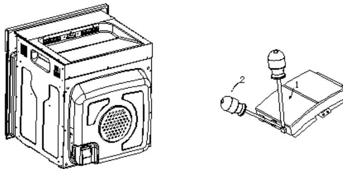
Move a screwdriver (1) slightly downwards (2) to open the box.
